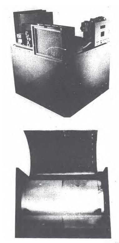
FIGURE 31.—Above, rotary cylinder dehumidifier used to control relative humidity in seed storage rooms; below, arrangement of cylinder, reactivation heaters, and seals in this dehumidifier. (Courtesy of Dryomatic Div.)
