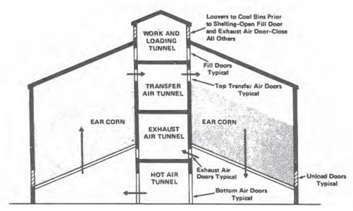
FIGURE 12.—Suction two-pass drying system. (Courtesy of Corn States Hybrid Serv., Des Moines, Iowa.)
