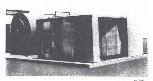
FIGURE 18.—High capacity rotary dehumidifier with 50,000 cubic-foot-per-minute airflow. Equipment includes a 150,000 cubic-foot-per-minute capacity main blower and air-heater unit. (Courtesy of Corr. States Hybrid Serv., Des Moines, Iowa.)
