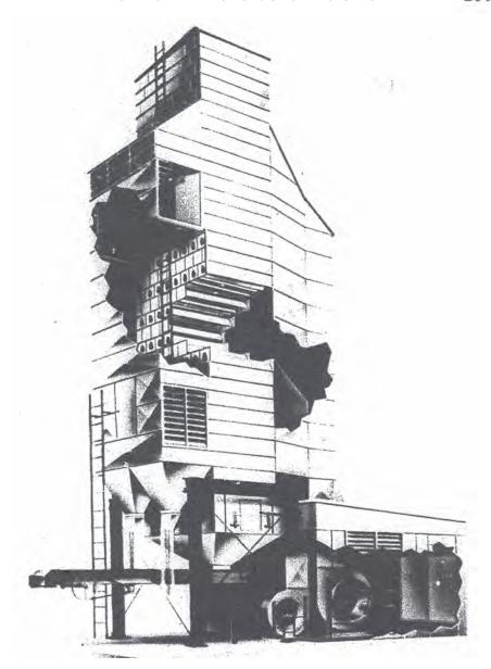
**FIGURE 13.**—Vertical continuous flow dryer. (Courtesy of Ferrell-Ross, Oklahoma City, Okla.)
