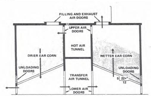
FIGURE 10.—Double- or two-pass drying system. (Courtesy of Corn States Hybrid Serv., Des Moines, Iowa.)
