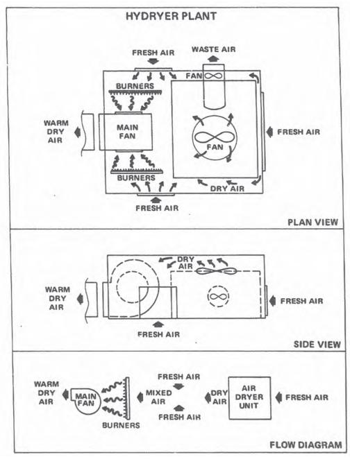
FIGURE 15.—Flow diagrams of air movement through a combination dehumidified-air heated-air dryer system. (Courtesy of Corn States Hybrid Serv., Des Moines, Iowa.)
