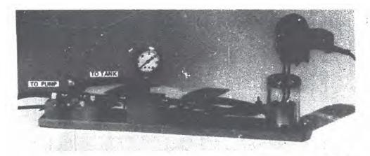
FIGURE 5.—Device for sealing tin cans from which air has been extracted by vacuum or gas has been added.
