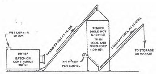
FIGURE 14.—Schematic flow diagram of dryeration process. (Courtesy of Coop. Ext. Serv., Purdue Univ.)
